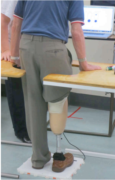
Figure 8: The interactive floor tiles in use in the Adelaide hospital, for a stepping task exercise.
