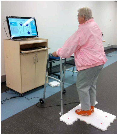
Figure 7: The interactive rehabilitation main tile in use for a balancing task.
