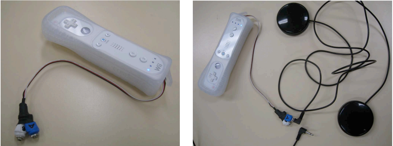
Figure 13 and 14. The modified WiiMote and switches that can be connected
