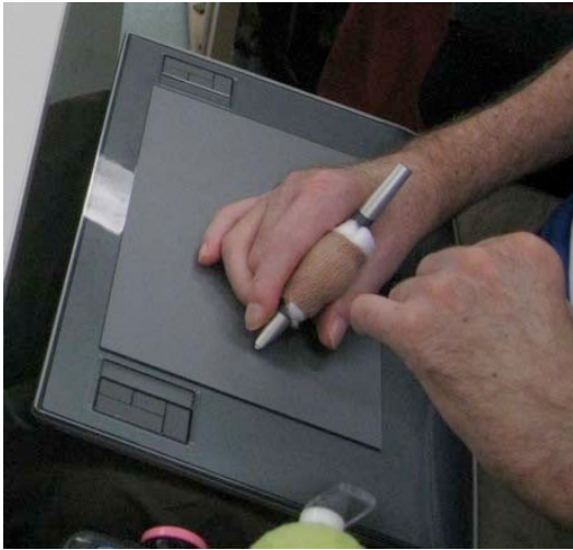
Figure 23 and 24. Using a Wacom tablet as an input device for a musical task, and a close-up of the modified pen for better grip.
