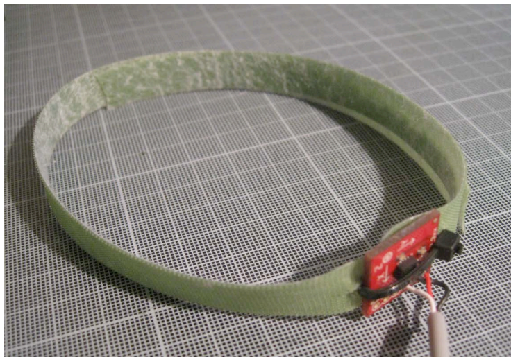
Figure 7. An accelerometer for motion sensing used in the project
