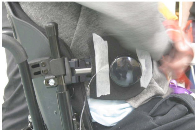
Figure 15. Wii game operated through an external switch operated by the elbow
