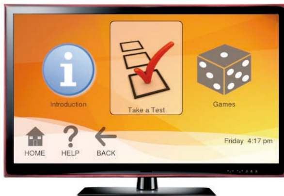
Figure 2. User interface for navigation through our Linux-based HTPC system for delivering step training program. Large, high contrast icons aid recognition for older adults with visual impairment. Dance mat arrows navigate left or right along menu items.
